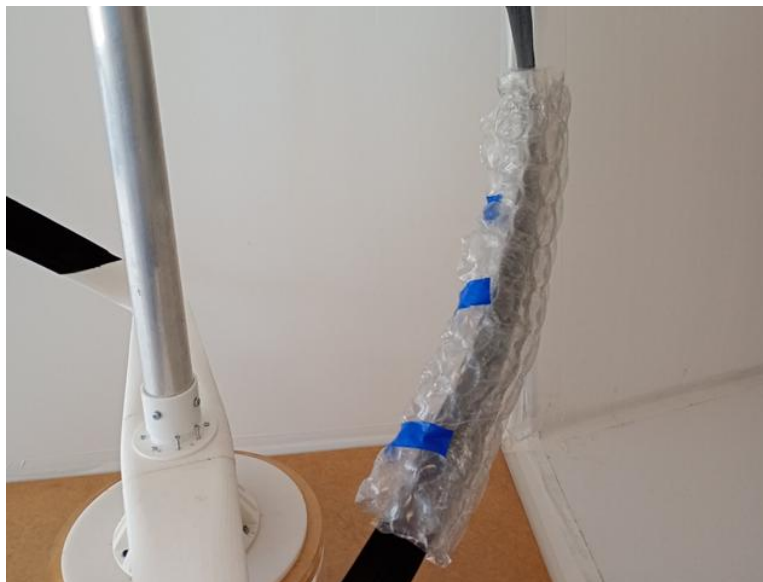
Figure 3.2: Example of induced anomaly during test - aerodynamic disturbance using bubble wrap on turbine blade.
